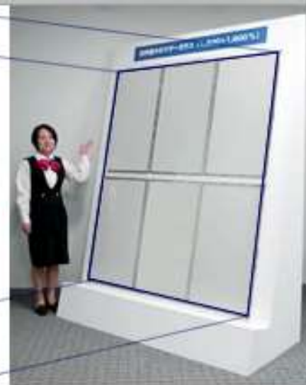
World's First* Large LCD Panel Production of a 1,500 x 1,800 mm Substrate. *As of June 2004
